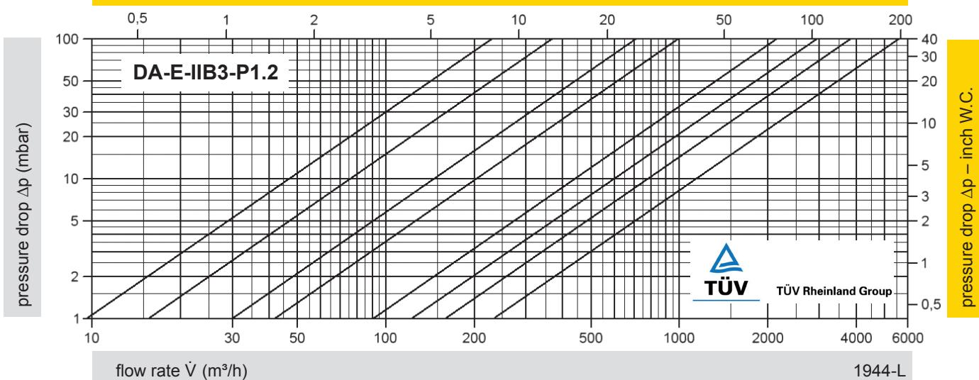
The flow capacity charts have been determined with a calibrated and TÜV certified flow capacity test rig.
