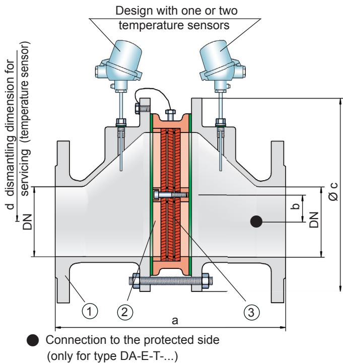
can be selected. The PROTEGO® DA-E series of flame arresters is available for explosion groups IIA to IIB3 (NEC Group D to C MESG  $\geq 0.65$  mm).
