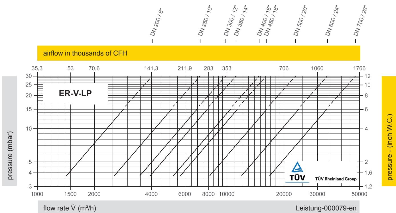
The flow capacity chart has been determined with a calibrated and TÜV certified flow capacity test rig.
