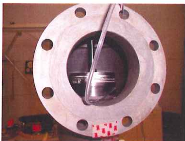
Figure 2: Location of test probe in EPA Method 21 test setup located directly at sealing surface
